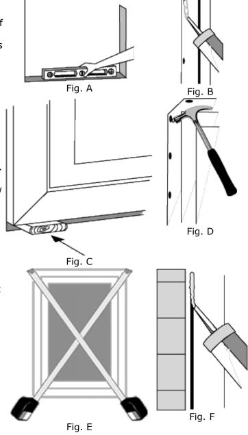
perimeter of the nailing fin aligned with pre-punched holes (Fig. B). After nailing the window in place and set for squareness, a house wrap tar type flashing tape is also required to seal the nailing fin on the exterior side of the fin covering the complete fin and exposed fasteners overlapping onto the project sheeting.
